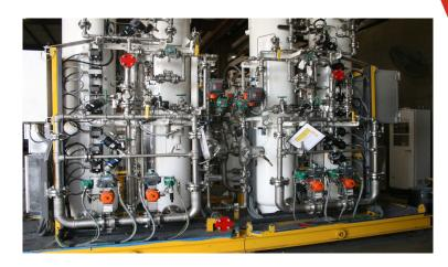
When compressed air enters the **GENERON®** system through coalescing filters, 99.999% of oil, water and liquid contaminates are removed. The filtered air is then directed by the solid state controller to the on-line tower where saturated air and water vapor adhere to the desiccant in a process called "adsorption".
