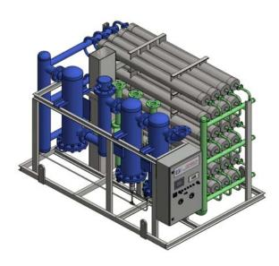
**GENERON®** Membrane separation systems are engineered and designed for efficient Nitrogen generation and mixed gas purification. The skid mounted systems are commonly used in the Oil & Gas Industry, Ammonia plants, Chemical Manufacturing Facilities, and Refineries. We build to standard designs or to custom engineering specifications to provide reliable, cost effective membrane separation solutions.
