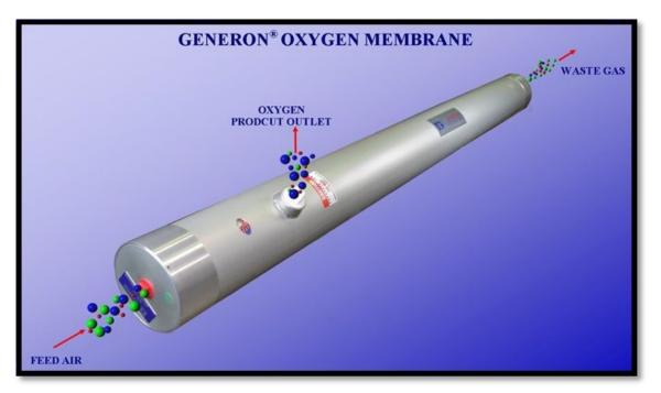
Membrane materials are formed into hollow fibers to provide a maximum surface area, for the high gas flow often required. **GENERON** holds over 100 U.S. patents on the design, packaging, and formulation of these hollow fiber membranes. The fibers are bundled into modules of various lengths and diameters to meet very specific flow rates and separation applications. Typical modules have anywhere from a half a million, to over a million fibers in one bundle
