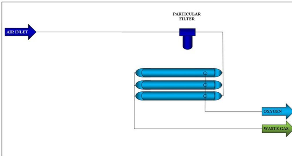
GENERON® Oxygen Membrane Modules are used in GENERON® Oxygen Generators, as well as supplied to approved OEM's for use in their proprietary systems.
