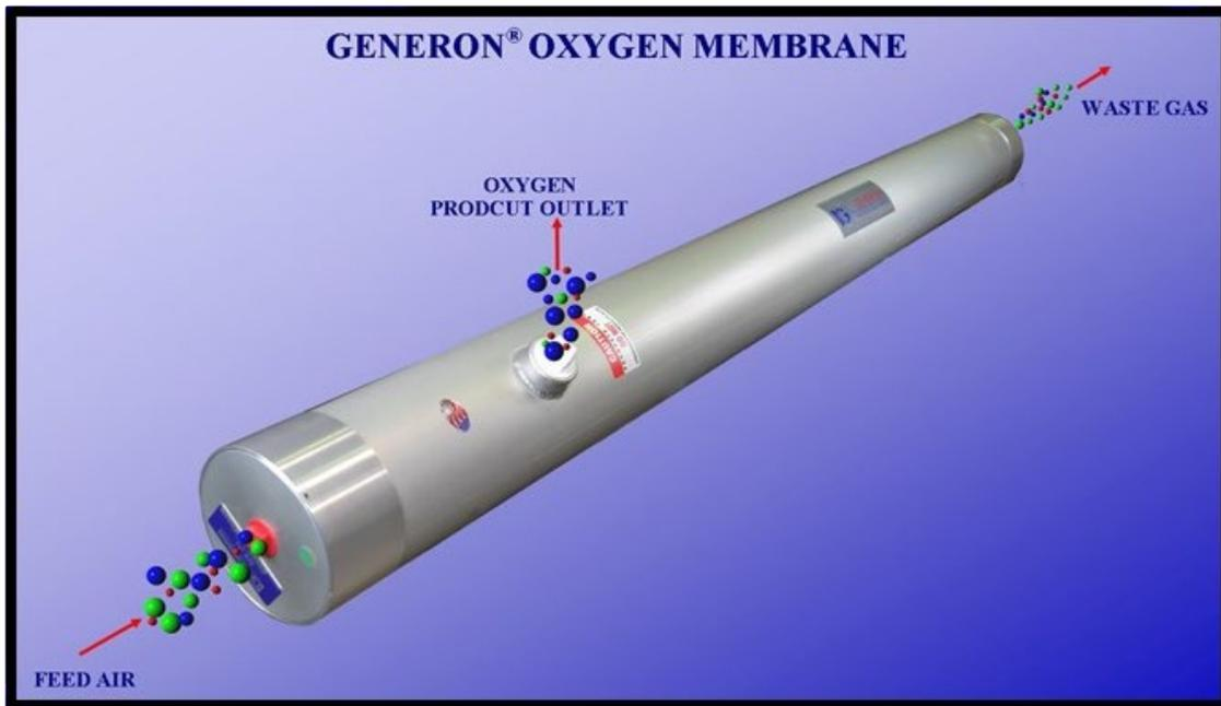
Membrane materials are formed into hollow fibers to provide a maximum surface area, for the high gas flow often required. **GENERON** holds over 100 U.S. patents on the design, packaging, and formulation of these hollow fiber membranes. The fibers are bundled into modules of various lengths and diameters to meet very specific flow rates and separation applications. Typical modules have anywhere from a half a million, to over a million fibers in one bundle
