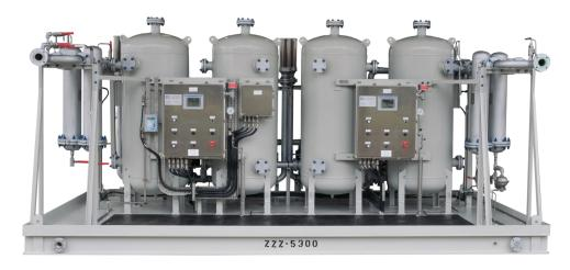
When compressed air enters the **GENERON®** system through coalescing filters, 99.999% of oil, water and liquid contaminates are removed. The filtered air is then directed by the solid state controller to the on-line tower where saturated air and water vapor adhere to the desiccant in a process called "adsorption".
