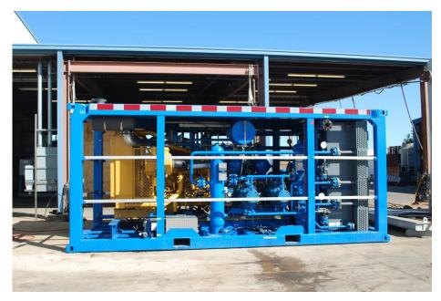
The compressor packages are built with removable roof panels to facilitate the removal of key equipment components, if required. Standardization of design and equipment are important considerations so units can be easily used by different drilling teams and maintenance personnel, as well as to achieve a standardization of spare parts inventory.
