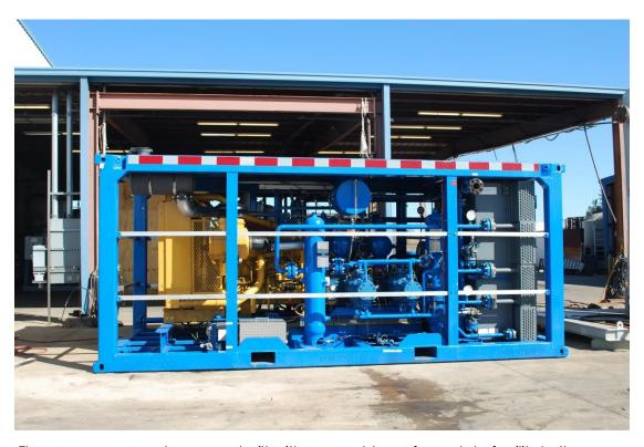
The compressor packages are built with removable roof panels to facilitate the removal of key equipment components, if required. Standardization of design and equipment are important considerations so units can be easily used by different drilling teams and maintenance personnel, as well as to achieve a standardization of spare parts inventory.
