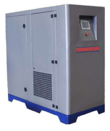
GENERON<sup>®</sup> Membrane Generators use patented high-efficiency membrane modules containing thousands of fibers. Compressed feed air is passed down the bores of the fibers at one end of the module with enriched nitrogen product gas exiting from the opposing end. Oxygen and water vapor are selectively removed from the feed air and vented as it flows to the other end of the module. These systems require low maintenance and less power to run.
