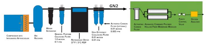
ISO 8573-1 2010: 1, 4, 1 used when ambient temperatures are above 50°F (PFD Diagram Above) ISO 8573-1 2010: 1, 2, 1 used when ambient temperatures are below 50°F
